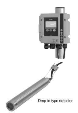
Detector options: Throw-in type and drop-in type Detectors are classified by installation conditions into two different types: throw-in type and drop-in type, the latter in which the detector is inserted into a long protection pipe that is 2 to 6 meters long.
